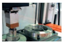
**EDM** Shapes in the surface of the punches are EDMed.
