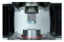
**Powder pressing** Top and bottom punches and the die plate are inserted into the press. The reference positions are provided by the precisely aligned chucks.
