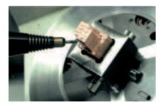
Milling Electrodes used to EMD the molds are machined on ITS system holders.
