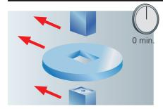
Pneumatically loosen die-plate and both punches.
