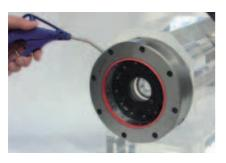
The chuck integrated with the machine spindle is opened with compressed air, either through an air-gun or through a fixed air supply.
