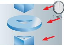
Insert and clamp new die-plate and punches.
