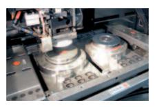
**Wire-EDM** The contours are produced on a WEDM center. The reference position is provided by the chuck.
