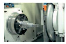
**Grinding** Punches may also be machined on cylindrical grinding machines.
