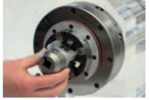
Any EROWA ITS system carrier can be clamped safely, quickly and precisely.
