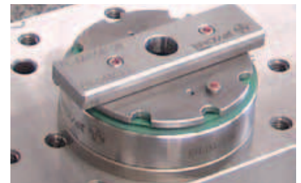
All axes, X, Y, Z and the center are checked with the same alignment plate.
